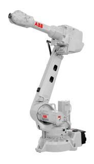
The IRB 2600 is the second model in the sharp generation range with enhanced and new capabilities. It is a compact robot with a high payload capacity. The design has been optimized for targeted applications like arc welding, material handling and machine tending. The IRB 2600 is available in three variants, with options for floor, wall, shelf, tilted or inverted mounting onfigurations.
