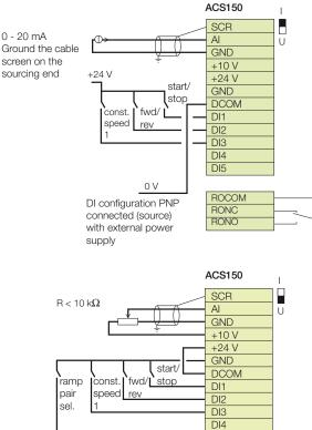
DI configuration NPN connected (sink)
