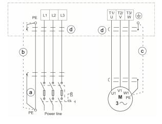
a. Two grounding conductors. Use two conductors if the cross-section of grounding conductor is less than 10  $\rm mm^2$  Cu or 16  $\rm mm^2$  Al (IEC/EN 61800-5-1). For example, use the cable shield in addition to the fourth conductor.
